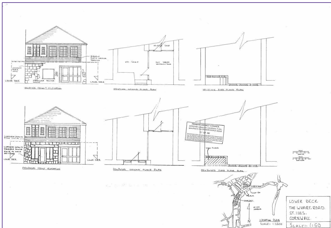
Planning drawing for installation of new shop front (02/P/0717 and 02/H/0088 of 2002). As existing at top and as proposed below) (Approved) .
