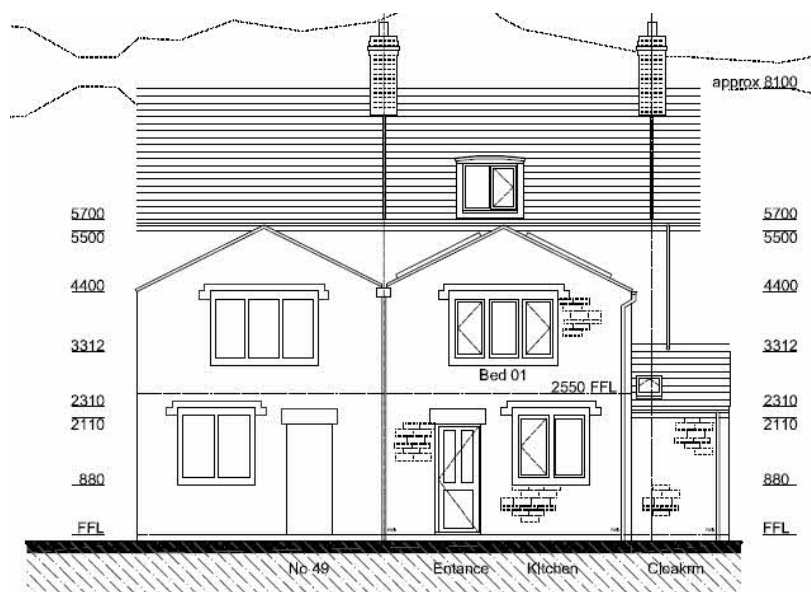
Proposed South Elevation showing revised inset glazing, and re-tiling of the two roofs and new solar panels.
