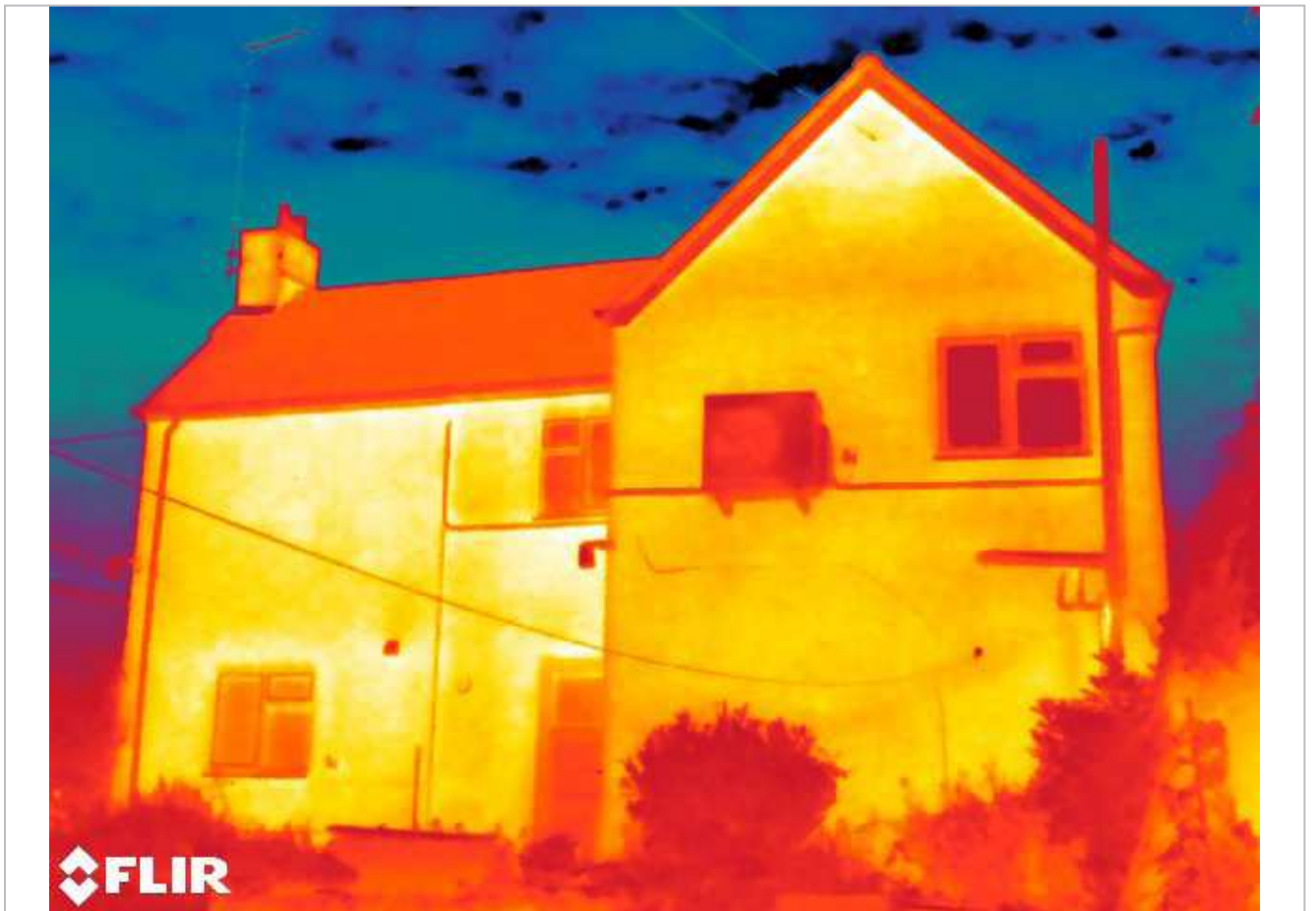
FLIR T540 (464 x 348 pixel resolution) with 42 degree lens = bat in flight detection distance of 51 m. Camera located 18 m from furthest point of building
