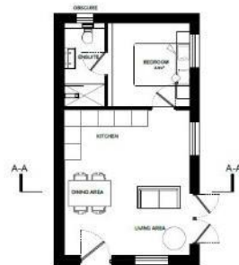
PROPOSED GROUND FLOOR-ANNEXE Total GIA-37.3m 2 (401sq.ft) Footprint-48.8m 2 Volume-169.2 m 3 Ridge/ Eaves- 17.0m/14.8m AOD
