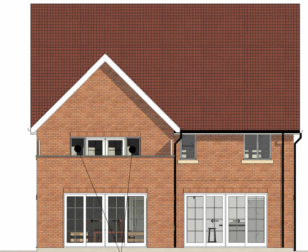
6 Rear Elevation - As-Built 1:100 Sidelights as built on site. Sidelights to have opening vents
