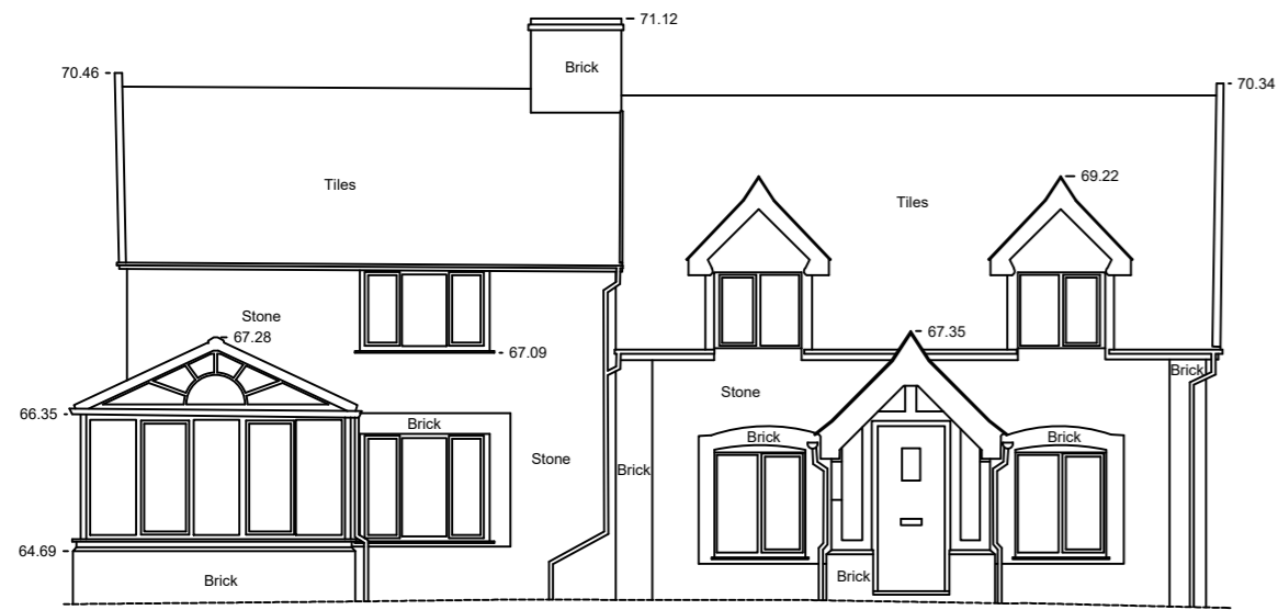
South West Elevation (Front) ▲ Datum line 63.00m
