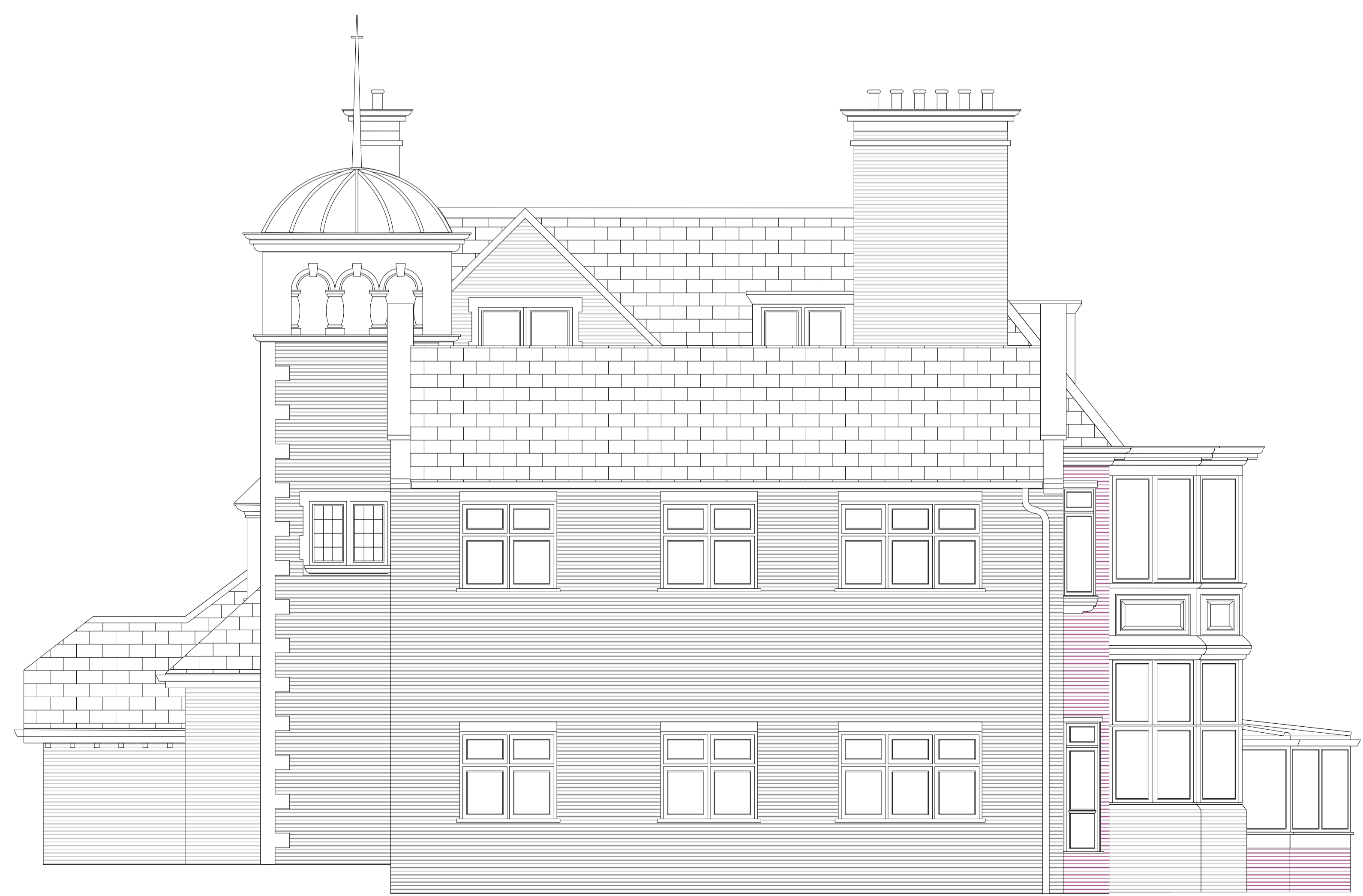
2 PROPOSED WEST ELEVATION Scale: 1:50 707 extent of new infill extension 1600 extent of new conservatory
