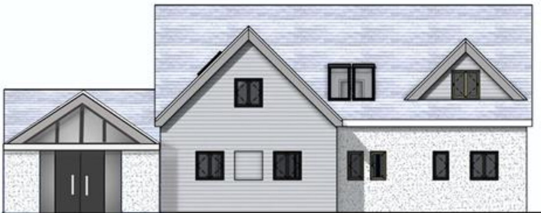
Proposed amendment to replace storage and recessed entrance with double entrance doors.
