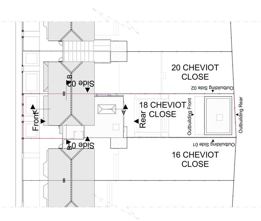
Proposed Site Plan Scale: 1:200 0 Status Scale @ A3 Purpose of Issue Originator Project Address Project Description Layout Title Express Planning Erection of a single-storey rear/side **S0** 1:200 18 Cheviot Close, Bexleyheath, Proposed Site Planning extension following the demolition of DA7 6SP **EXPRESS** Proposed Site Plan Project No: Date Checked by existing extensions and erection of a PLANNING single-storey outbuilding (summer 178-DA7 06 February 2024 MA house)
