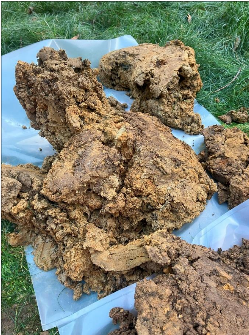
Figure 4-E: A photograph of the River Terrace Deposits encountered in trial pit S1-TP01
