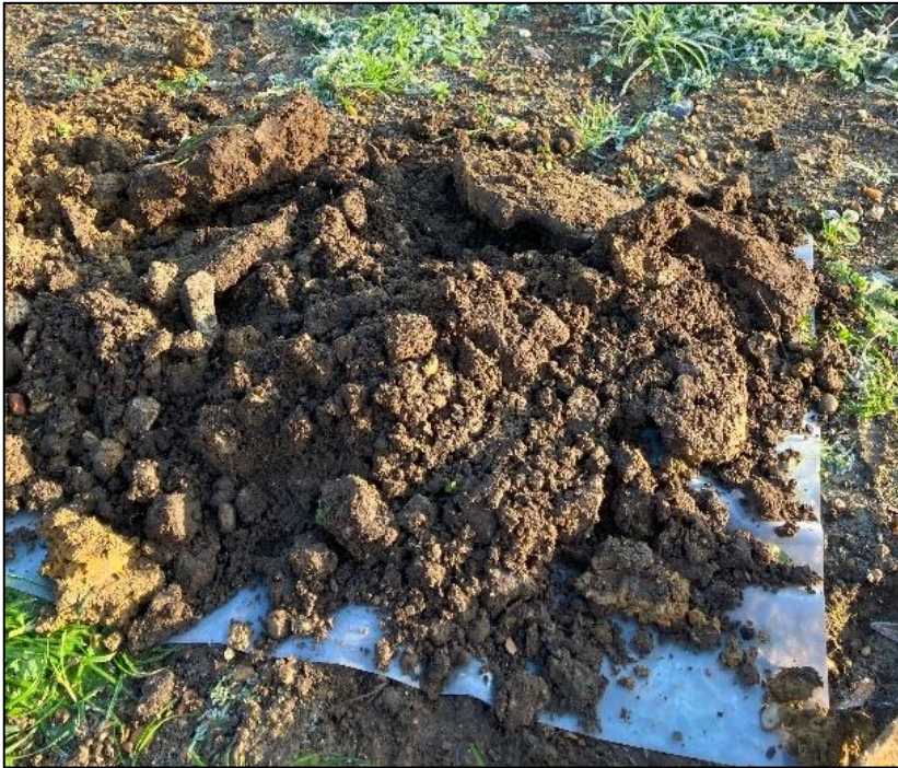
Figure 4-B: Photograph of the Topsoil - Made Ground deposits encountered in S1-TP02
