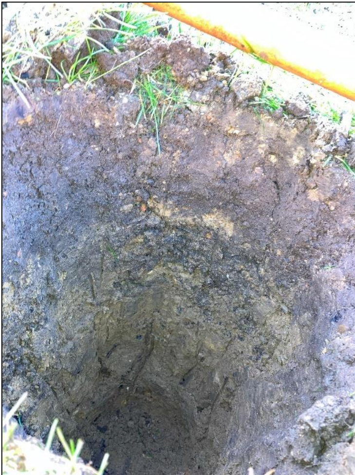
Figure 4-C: Photograph of the Topsoil - Made Ground deposits encountered in S1-TP03
