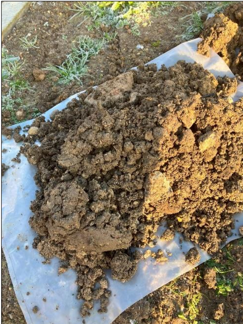
Figure 4-D: A photograph of the typical Made Ground encountered on site
