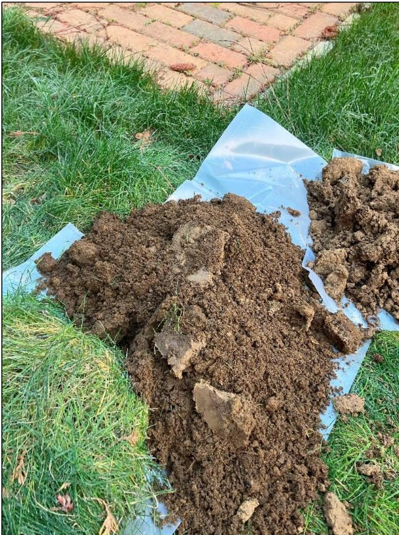
Figure 4-A: Photograph of the Topsoil deposits encountered from S1-TP01
