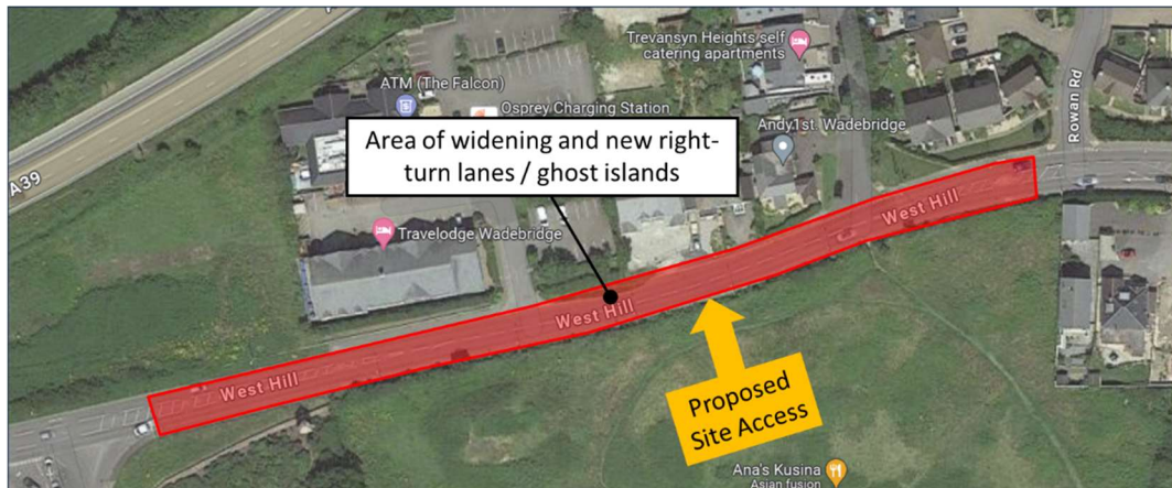
Figure 4.1 – Proposed Area of Widening and Right-turn Lanes / Ghost Islands on West Hill
