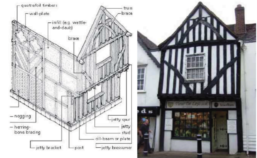
TYPICAL JETTIED TIMBER FRAME
