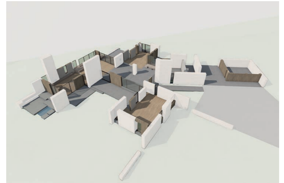
2 - The floor plates step down with the natural contours of the land to provide level terraces into the garden. Doors and large format glazing provide access and help to draw the landscape into the building with the timber panel infill elements positioned to frame long views into the landscape but also long views through the building itself.
