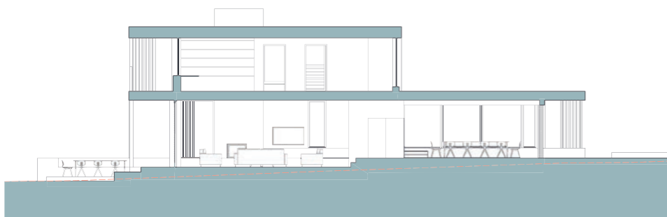
Building steps with the natural contours of the existing site, minimising cut and fill.
