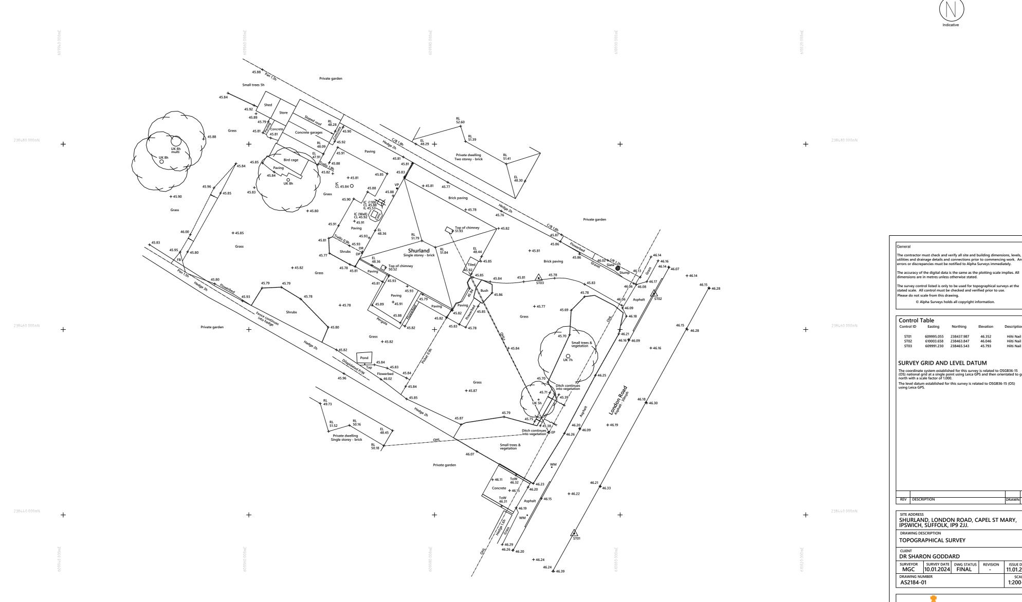
The contractor must check and verify all site and building dimensions, levels, utilities and drainage details and connections prior to commencing work. Any errors or discrepancies must be notified to Alpha Surveys immediately.
