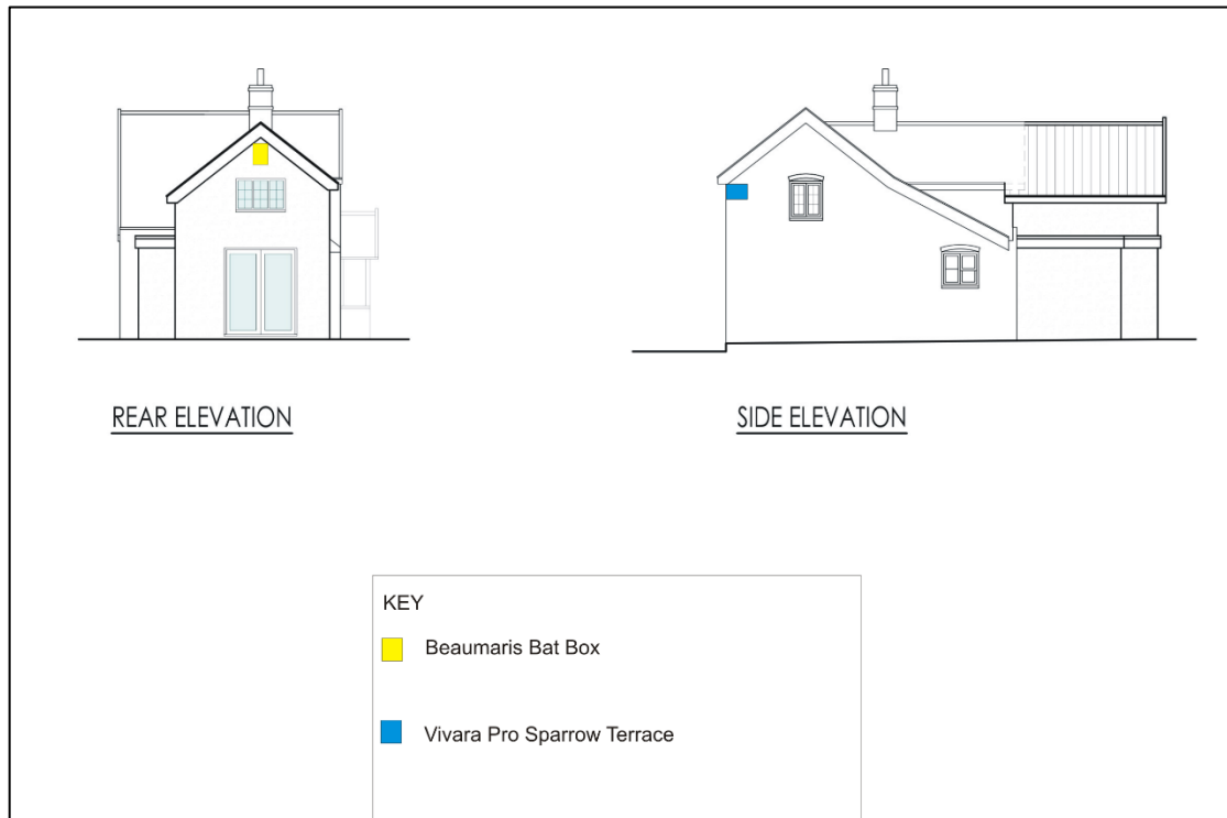
Figure 1: Recommended locations for habitat enhancements.
