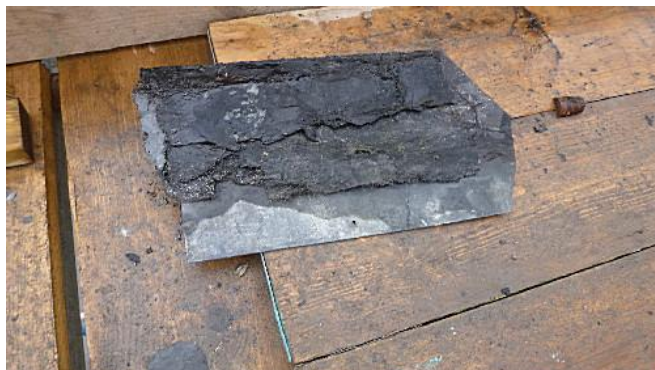
Fibre cement slate with reinforced bitumen coating
