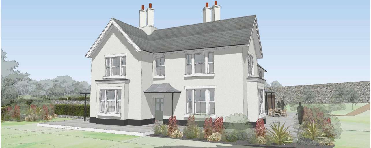
Fig. 11. Proposed new side elevation with additional window opening and pre-existing front door redefined as a side access door
