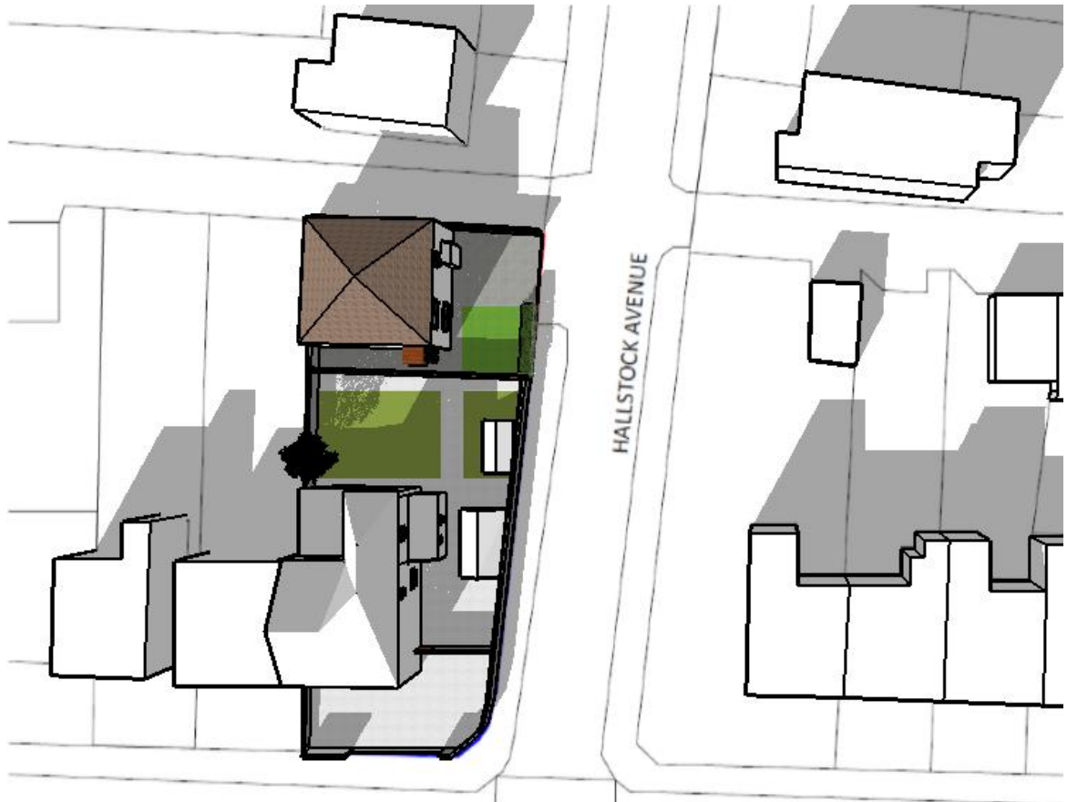
Figure 6.2: Proposed Aerial View of the Proposed development demonstrating the shadowing of the proposed building and nearby properties
