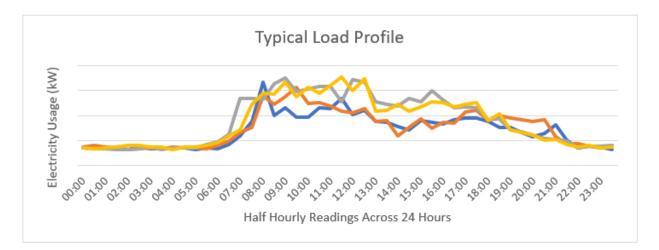
The PV scheme has been designed to account for the anticipated peak usage with additional consideration for the potential future provision for electric vehicle charging onsite. It should be noted that the installation can be extended in the future, should it be appropriate to do so.
