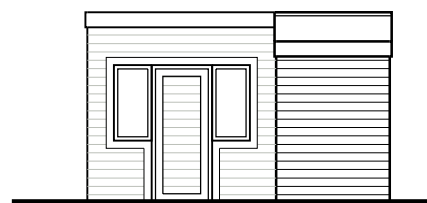
TYPICAL GARDEN STORAGE BUILDING PROPOSED TO REAR - TO BE WITHIN PERMITTED DEVELOPMENT LIMITS (NOT MORE THAN 2.5M TALL IF WITHIN 2M OF ADJACENT BOUNDARIES)
