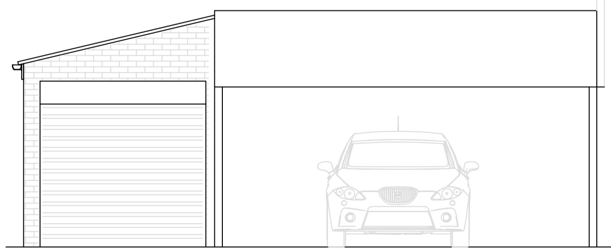
REAR WEST ELEVATION EXISTING - SCALE 1:50
