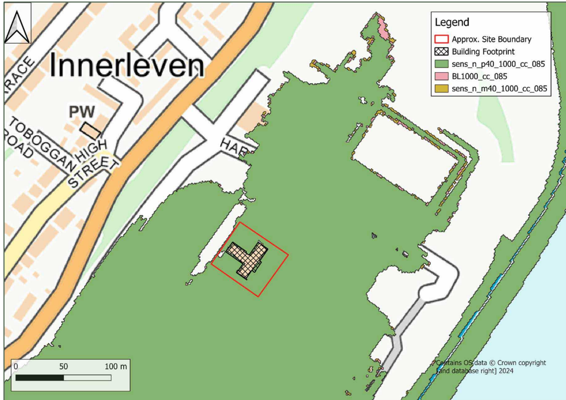
Figure 5-17 –1:1000 (0.1% AEP) plus CC Sensitivity testing of Mannings n roughness
