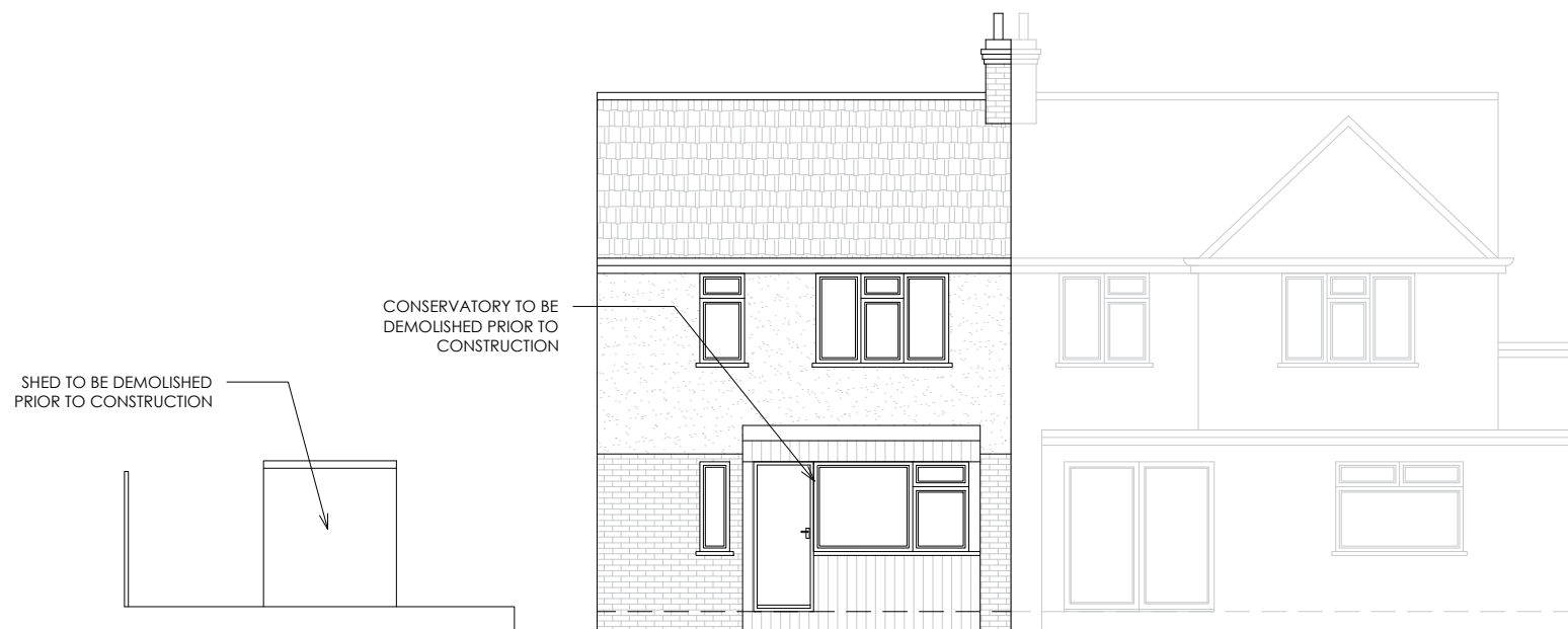
EXISTING REAR ELEVATION 1:100
