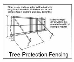
This is to be provided by Braced Heras Fencing or solid panels. Post-holes shall be excavated by powered hand auger or low ground-pressure plant working of ground protection or outside the Precautionary Zone. Alternative more traditional post supports such as the Heras Steadfast system with an additional brace can be used where this can be pinned into position and fitted with an Anti-Tamper Coupler.
