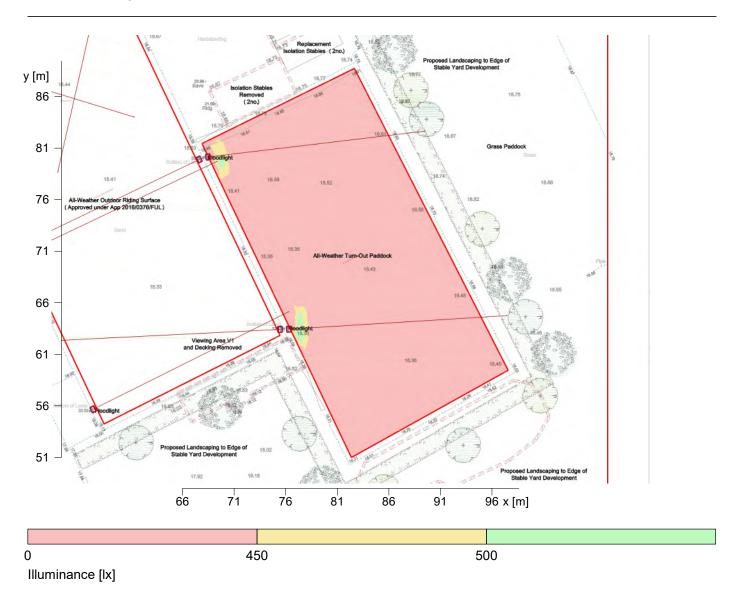
Height reference plane Average illuminance Minimum illuminance Maximum illuminance Uniformity U<sub>o</sub> Diversity U<sub>d</sub>  $\begin{array}{ccc} & : 0.00 \text{ m} \\ \overline{\text{E}}_{\text{m}} & : 153 \text{ lx} \\ \overline{\text{E}}_{\text{min}} & : 38 \text{ lx} \\ \overline{\text{E}}_{\text{max}} & : 513 \text{ lx} \end{array}$
