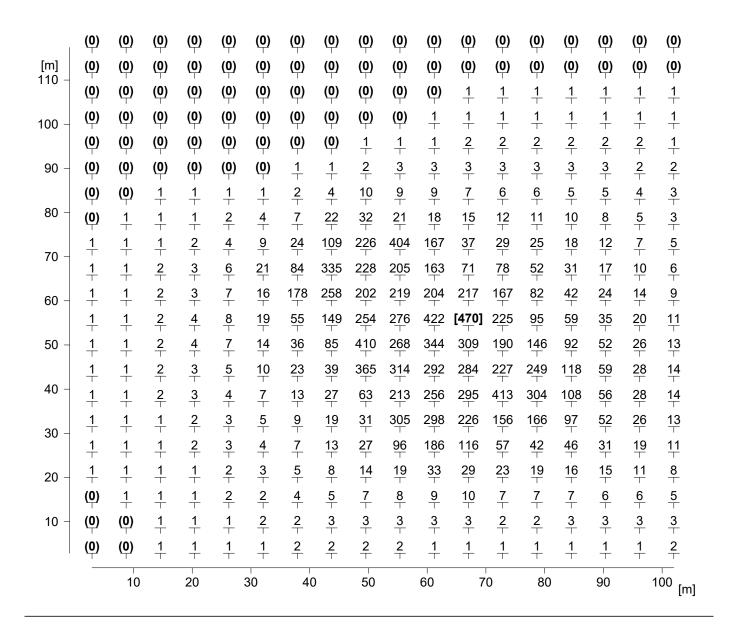
Height reference plane Average illuminance Minimum illuminance Maximum illuminance Uniformity U<sub>o</sub> Diversity U<sub>d</sub>  $\begin{array}{ccc} & : 0.00 \text{ m} \\ \overline{\text{E}}_{\text{m}} & : 39 \text{ lx} \\ \overline{\text{E}}_{\text{min}} & : 0 \text{ lx} \\ \overline{\text{E}}_{\text{max}} & : 470 \text{ lx} \end{array}$
