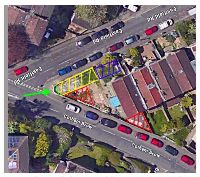
The yellow hatched area is a temporary graded hard standing driveway to allow construction vehicles and deliveries to occur without disruption to traffic.
