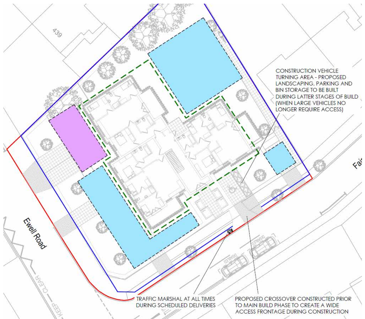
Figure 4.2: Construction Site Setup – Main Build Phase
