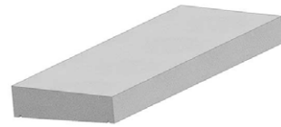
② Portland stone coping example (colour not indicative of final product - for information only) - size and profile to match existing
