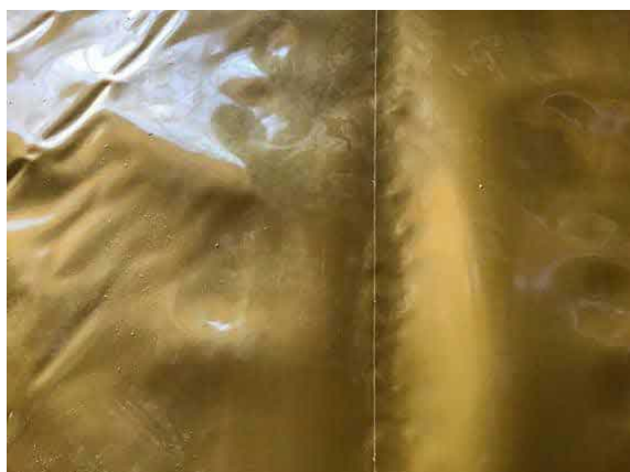
Plot 4 hand welded membrane lap.
