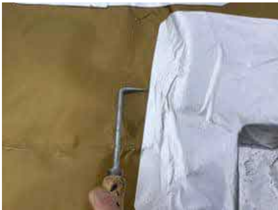
Plot 5 pick testing all SAGM detailing.
