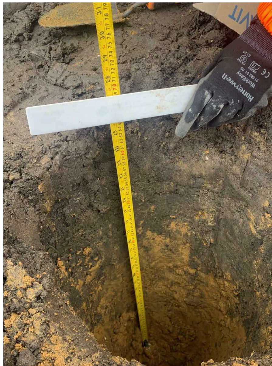
Photo 3: Plot 28 Rear garden showing the depth of topsoil and subsoil and the geotextile.
