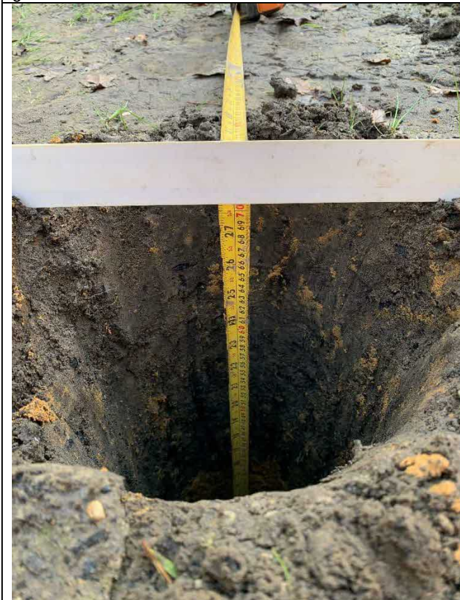
Photo 11: Plot 67 rear garden showing depth to geotextile.
