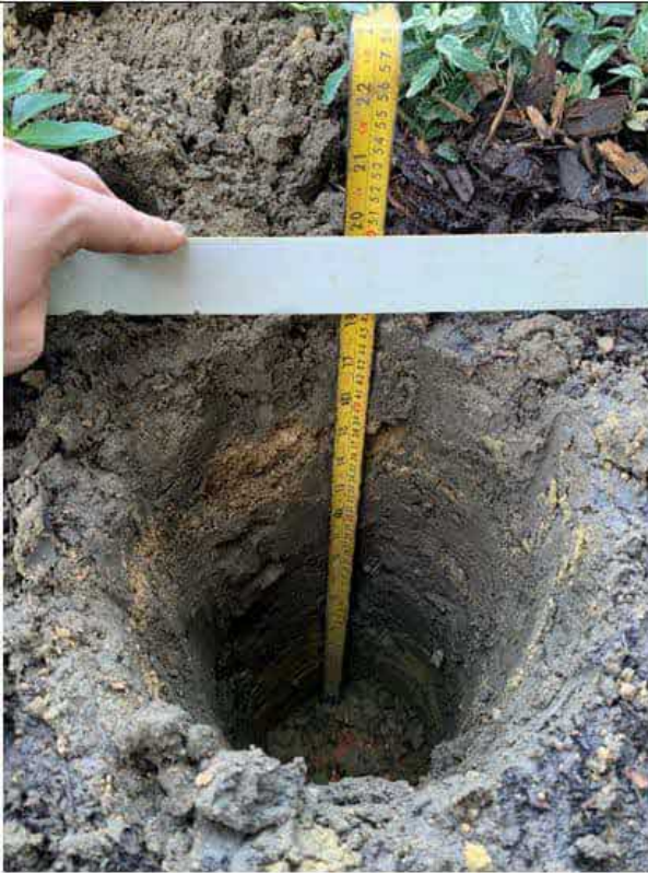
Photo : Plot 64 front garden showing depth to geotextile.
