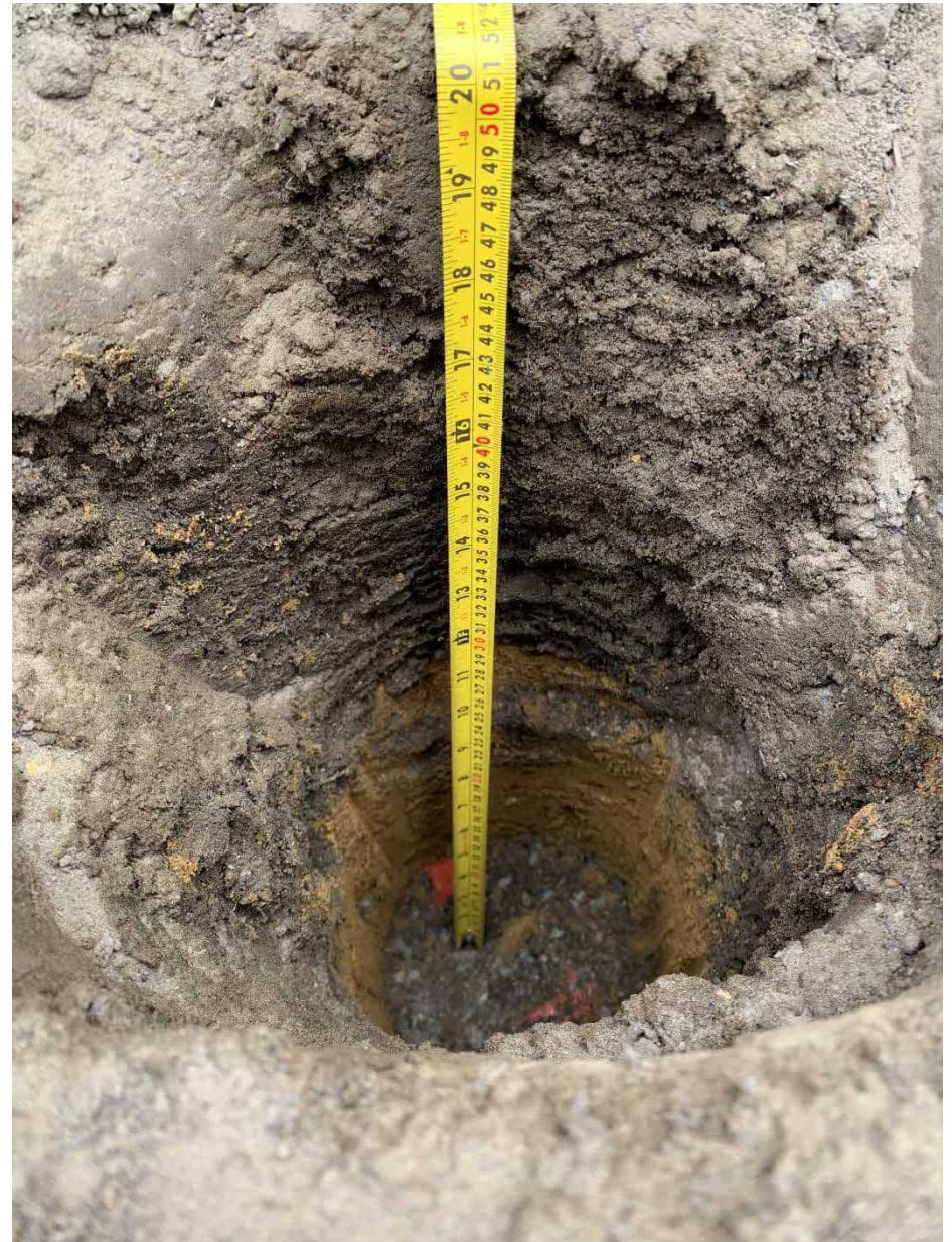
Photo 2: Plot 37 Front garden showing topsoil, subsoil and geotextile.
