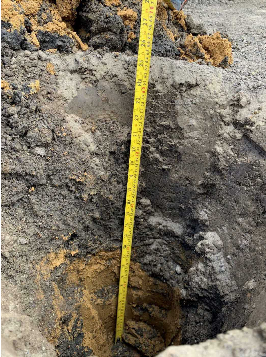
Photo 1: Plot 36 Front Garden showing topsoil, subsoil and geotextile.
