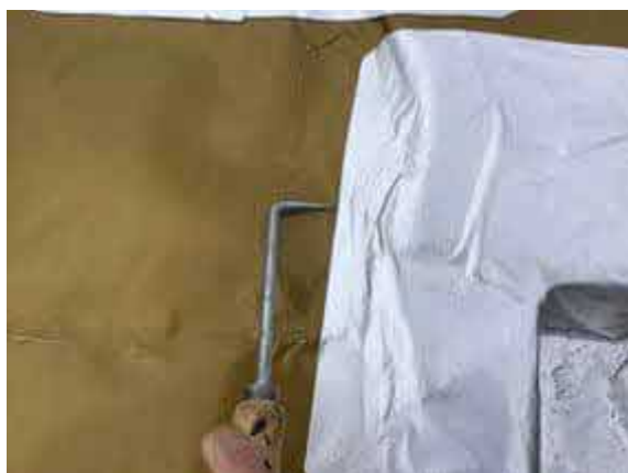
Plot 5 pick testing all SAGM detailing.
