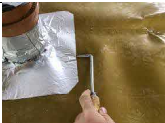
Pick testing all SAGM detailing.
