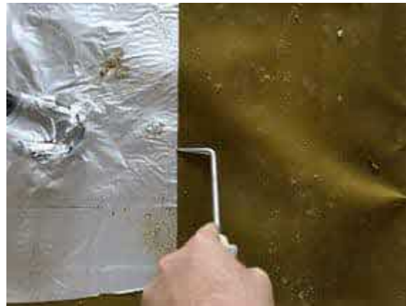
Pick testing all SAGM detailing.
