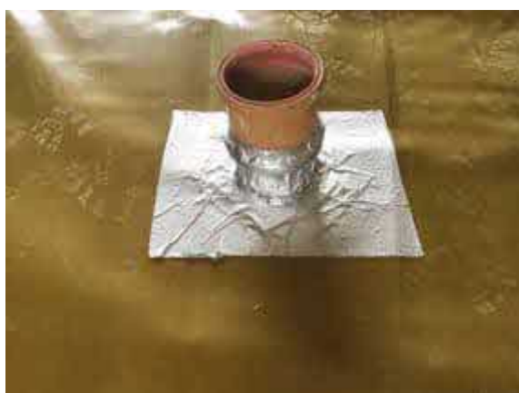
Plot 6 typical pipe penetration seal using SAGM.
