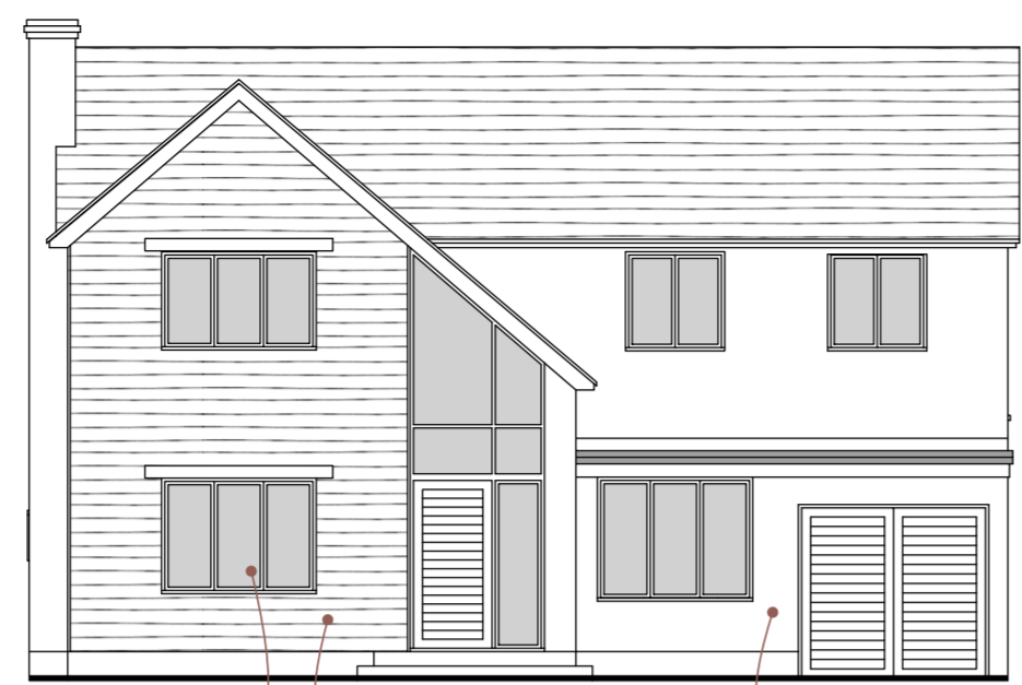
powder-coated grey aluminium windows and doors horizontal composite cladding painted off-white render NORTH / FRONT ELEVATION
