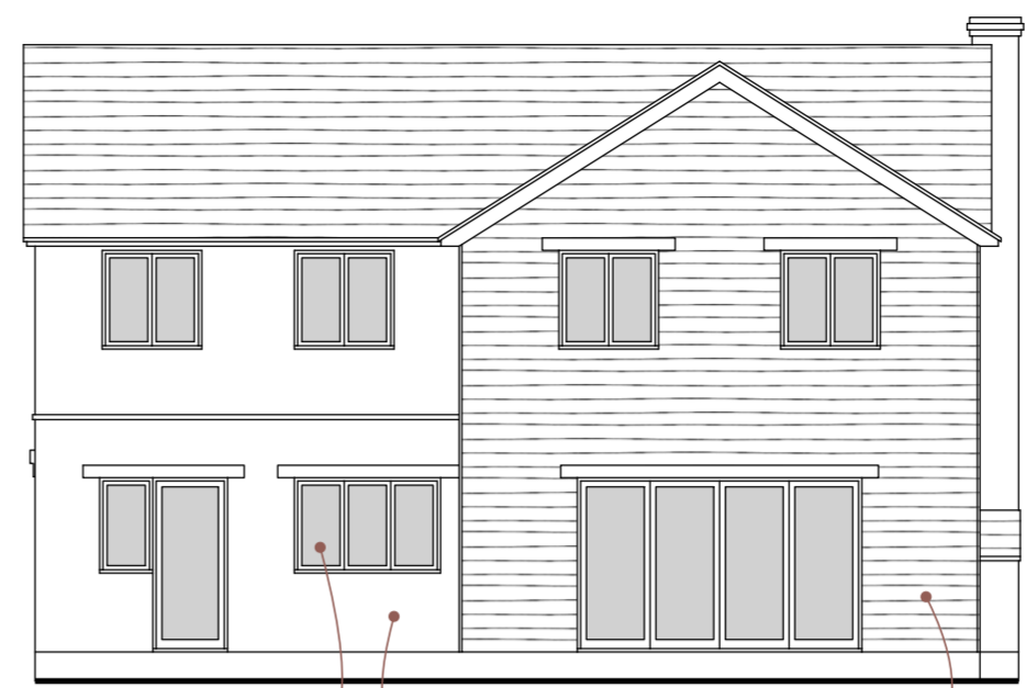
powder-coated grey aluminium windows and doors painted off-white render horizontal composite cladding SOUTH / REAR ELEVATION
