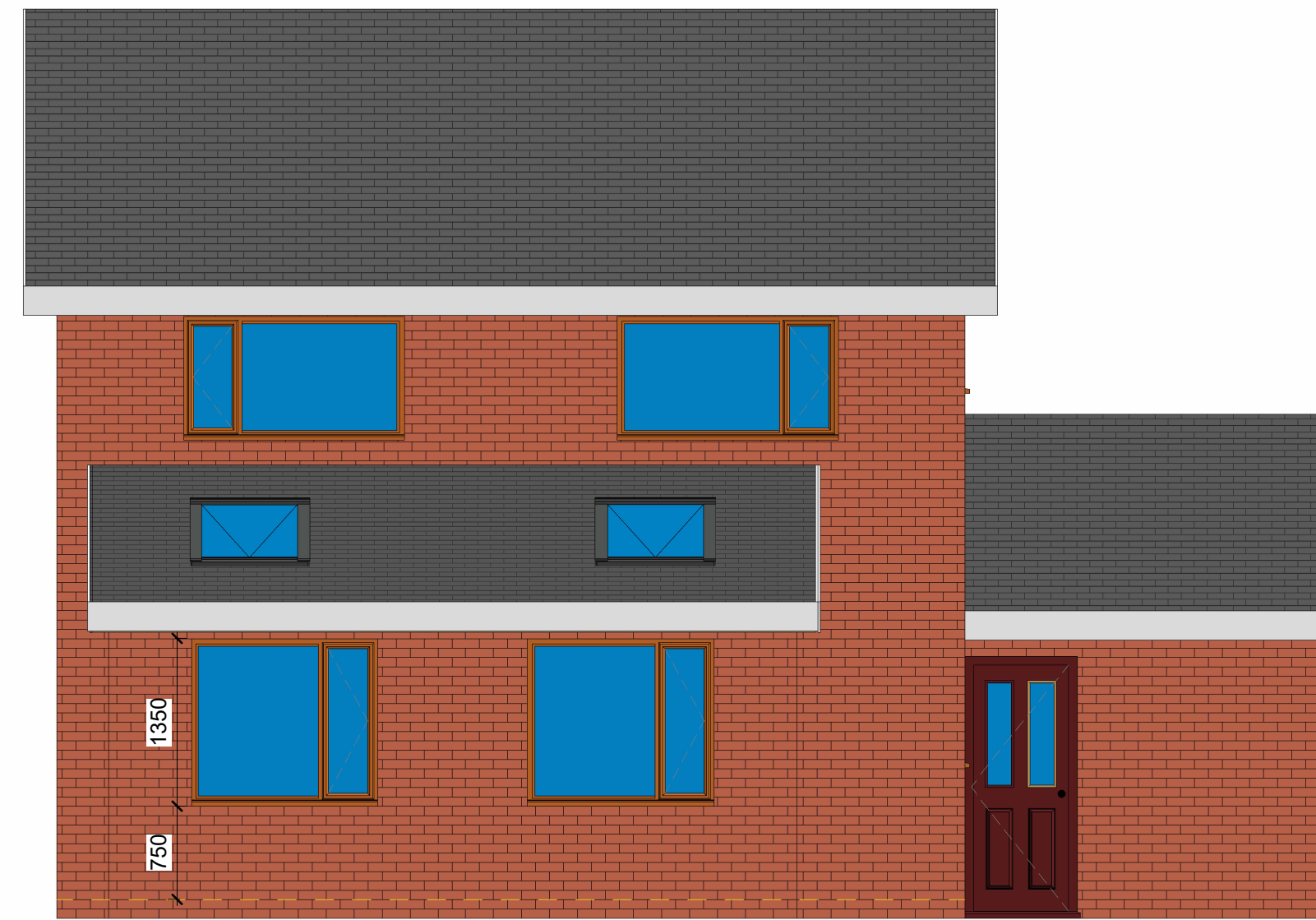
4 Proposed Rear Elevation 1 : 50
