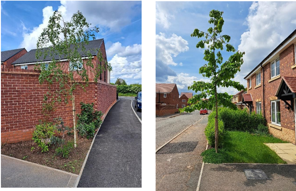
Figure 4 Poor planting practices to avoid: Restricted rooting volumes, impermeable surfacing and planting trees near underground services/drainage runs
