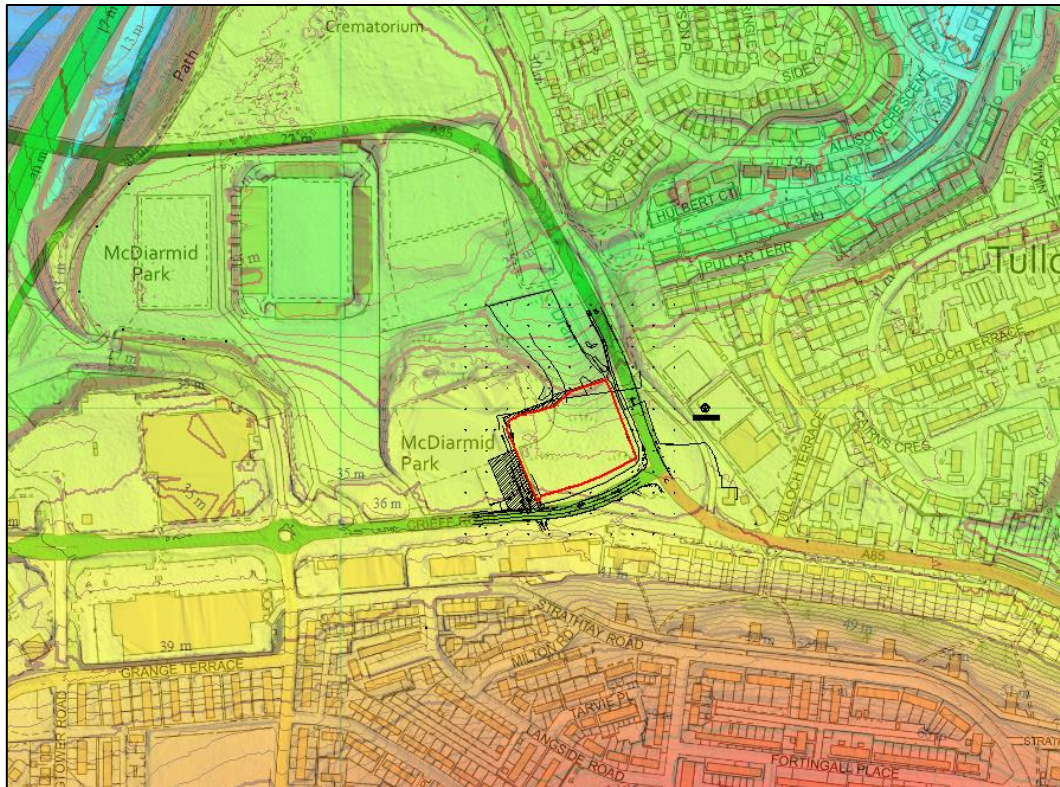
Figure 3: Site topography created from the LiDAR data with 1m contour lines added and selected heights labelled (m AOD).
