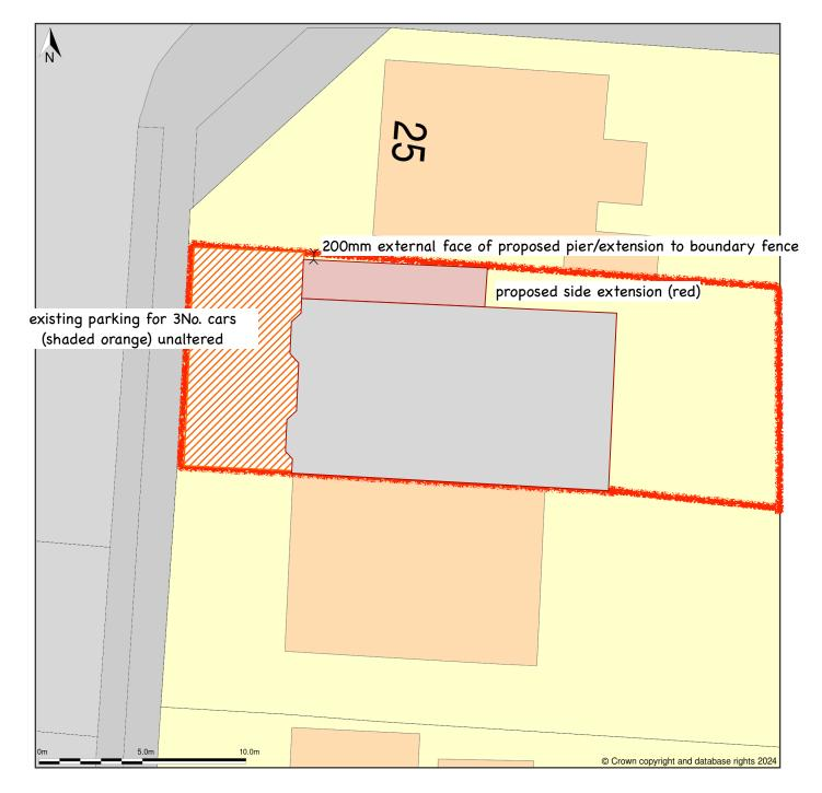
Site Plan (also called a Block Plan) shows area bounded by: 468059.49, 107537.34 468095.49, 107573.34 (at a scale of 1:200), OSGridRef: SU6807 755. The representation of a road, track or path is no evidence of a right of way. The representation of features as lines is no evidence of a property boundary.
