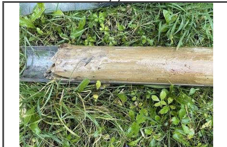
Photo OE/1702/1057/R3/P06 – Window Sample WS1 – Drilling cores 1.0 to 1.3m bgl – Natural orange CLAY.
