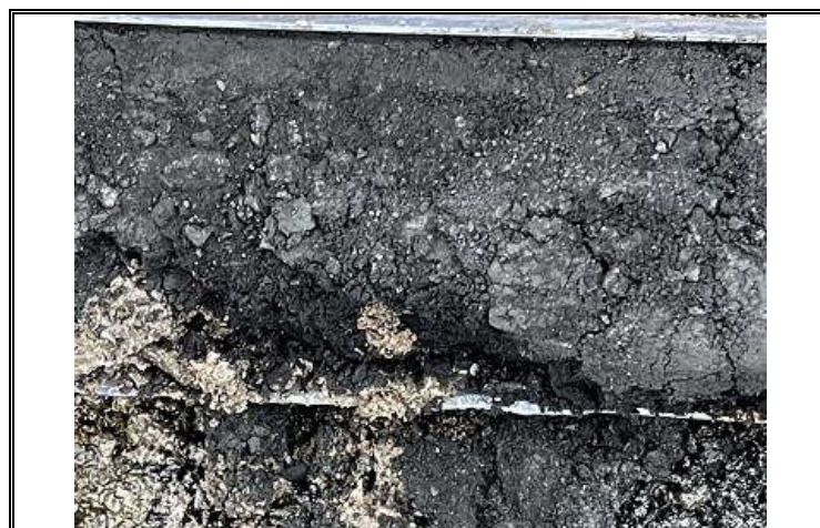
Photo OE/1702/1057/R3/P30 – Window Sample WS5 – Drilling cores 2.3 to 2.4m bgl –Coal seam.
