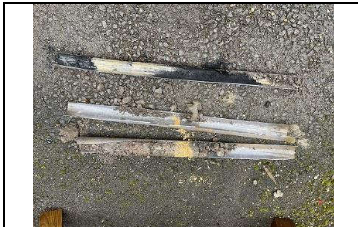
Photo OE/1702/1057/R3/P23 – Window Sample WS5 – Drilling cores at 0.0 to 3.0m bg – poor receoryl.
