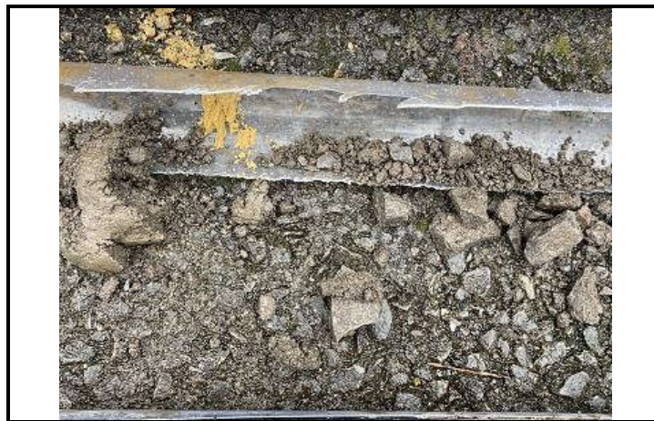
Photo OE/1702/1057/R3/P27 – Window Sample WS5 – Drilling cores 1.0 to 1.5m bgl – Made Ground – rock fill poor recovery.
