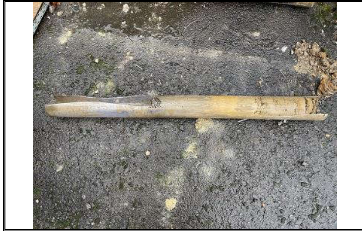
Photo OE/1702/1057/R3/P13 – Window Sample WS2 – Drilling cores 1.0 to 1.6m bgl – Natural orange CLAY.
