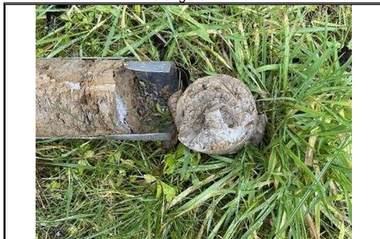
Photo OE/1702/1057/R3/P09 – Window Sample WS1 – Drilling core at 1.9m bgl – Very stiff weathered Mudstone.
