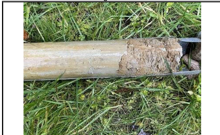
Photo OE/1702/1057/R3/P08 – Window Sample WS1 – Drilling cores 1.7 to 1.9m bgl – Natural orange CLAY.
