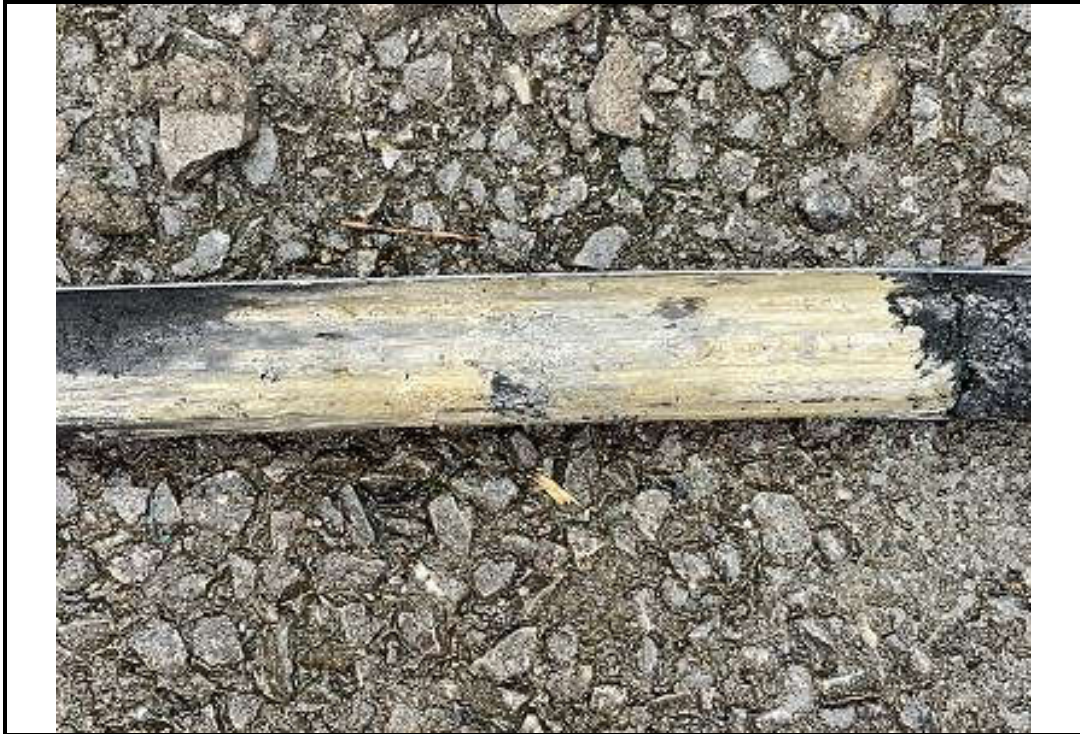
Photo OE/1702/1057/R3/P31 – Window Sample WS5 – Drilling cores 2.7 to 2.9m bgl –Soft natural Clay.
