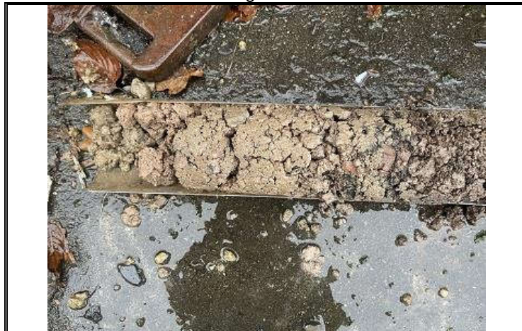
Photo OE/1702/1057/R3/P14 – Window Sample WS2 – Drilling cores 0.0 to 0.3m bgl – Made Ground – rock fill.
