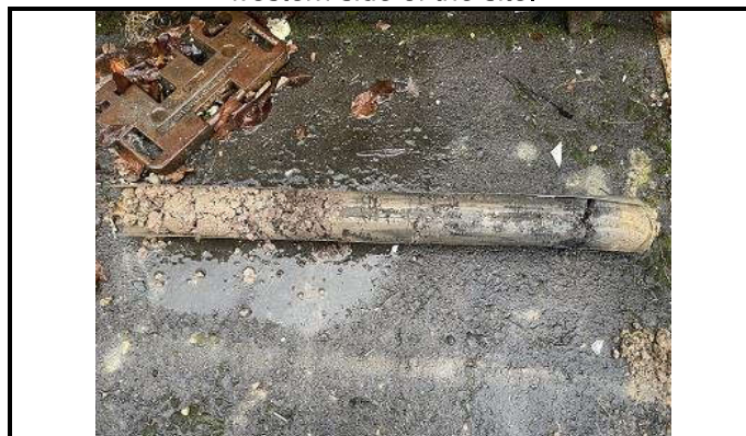
Photo OE/1702/1057/R3/P12 – Window Sample WS2 – Drilling cores 0.0 to 0.9m bgl – Made Ground.
