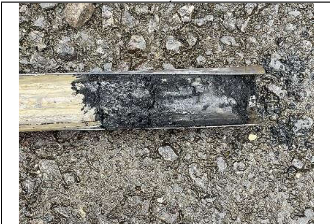
Photo OE/1702/1057/R3/P32 – Window Sample WS5 – Drilling cores 2.9 to 3.0m bgl –Coal seam before encountering hard weathered Mudstone..
