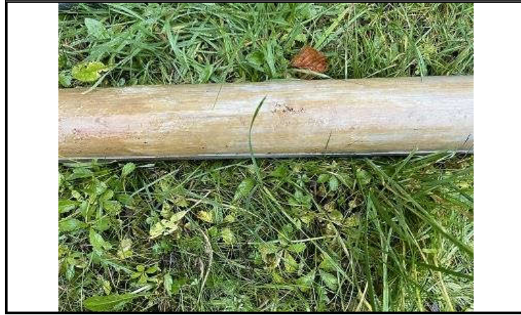
Photo OE/1702/1057/R3/FP07 – Window Sample WS1 – Drilling cores 1.3 to 1.7m bgl – Natural orange CLAY.
