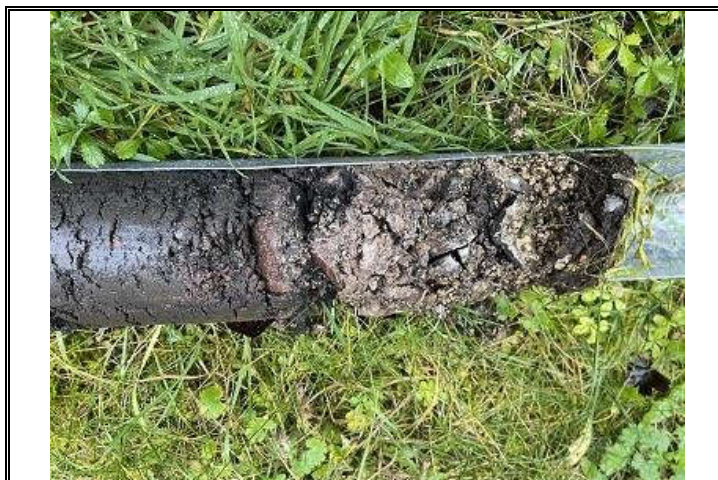
Photo OE/1702/1057/R3/P03 – Window Sample WS1 – Drilling cores 0.0 to 0.19m bgl – turf/topsoil/rock fill.
