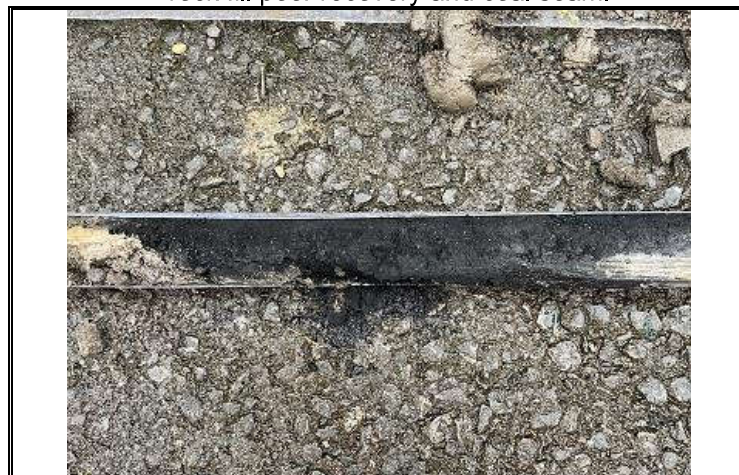
Photo OE/1702/1057/R3/P29 – Window Sample WS5 – Drilling cores 2.3 to 2.6m bgl –Coal seam.
