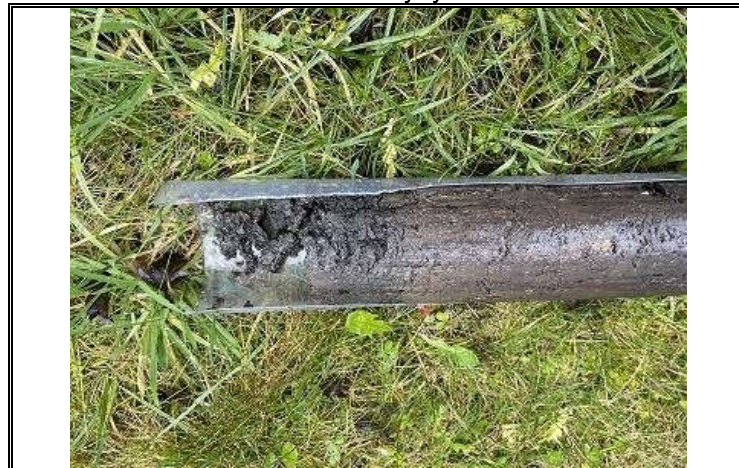
Photo OE/1702/1057/R3/P05 – Window Sample WS1 – Drilling cores 0.7 to 1.0m bgl – Made Ground clayey fill.
