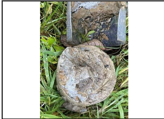
Photo OE/1702/1057/R3/P10 – Window Sample WS1 – Drilling core at 1.9m bgl – Very stiff weathered Mudstone.
