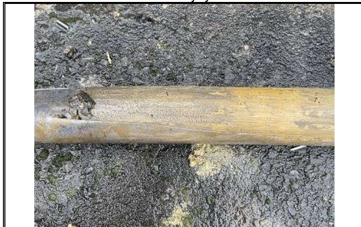
Photo OE/1702/1057/R3/P17 – Window Sample WS2 – Drilling cores 0.9 to 1.6m bgl – Natural soft orange CLAY
