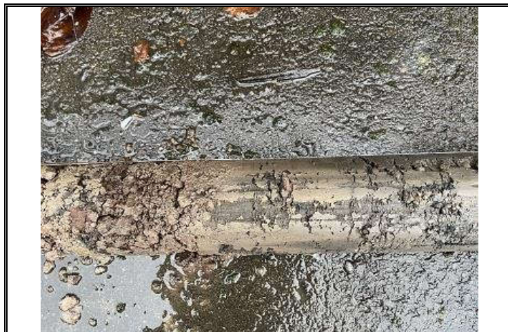
Photo OE/1702/1057/R3/15 – Window Sample WS2 – Drilling cores 0.3 to 0.6m bgl – Made Ground – soft clayey fill.
