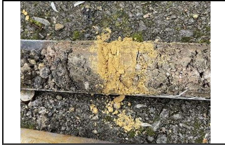
Photo OE/1702/1057/R3/P25 – Window Sample WS5 – Drilling cores 0.2 to 0.3m bgl – Made Ground – Crushed Sandstone.
