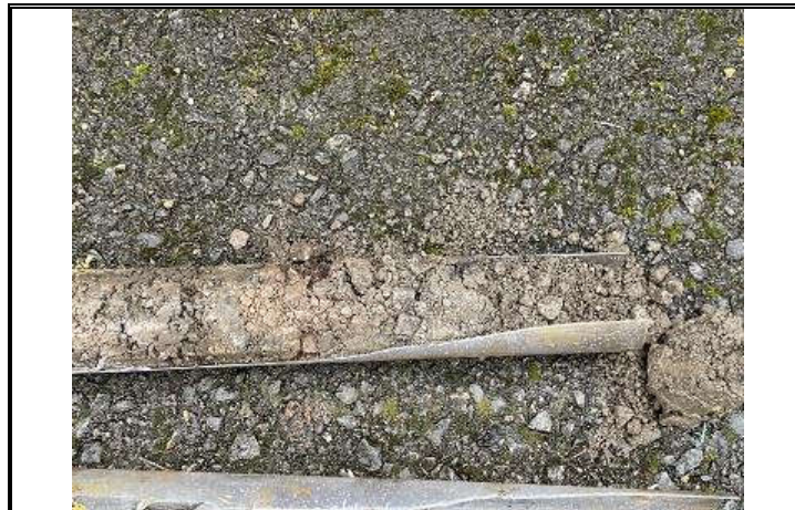
Photo OE/1702/1057/R3/P26 – Window Sample WS5 – Drilling cores 0.3 to 1.0m bgl – Made Ground – rock fill.
