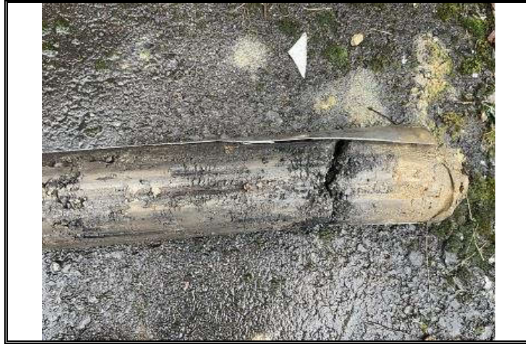
Photo OE/1702/1057/R3/P16 – Window Sample WS2 – Drilling cores 0.6 to 0.9m bgl – Made Ground – soft clayey fill.
