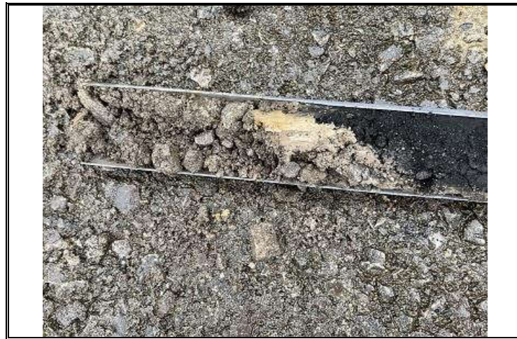
Photo OE/1702/1057/R3/P28 – Window Sample WS5 – Drilling cores 2.2 to 2.3m bgl – Made Ground – rock fill poor recovery and coal seam.
