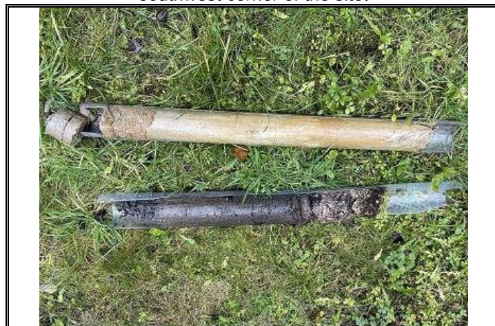
Photo OE/1702/1057/R3/P02 – Window Sample WS1 – Drilling cores 0.0 to 1.9m bgl.
