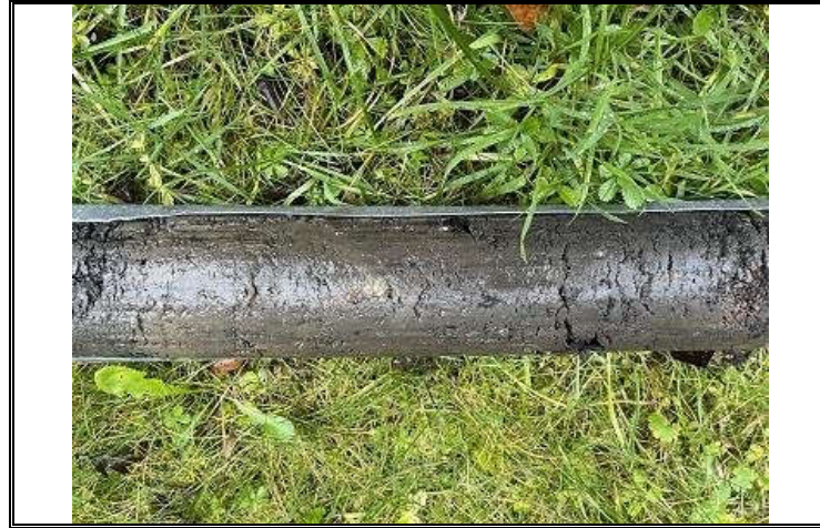
Photo OE/1702/1057/R3/P04 – Window Sample WS1 – Drilling cores 0.19 to 0.7m bgl – Made Ground clayey fill.
