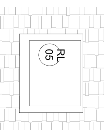
Proposed roof windows: Top Hung grey colour framed roof windows Product ref: VELUX www.velux.co.uk/products/roof-windows/single-roof-windows/standard-single-roof-window
