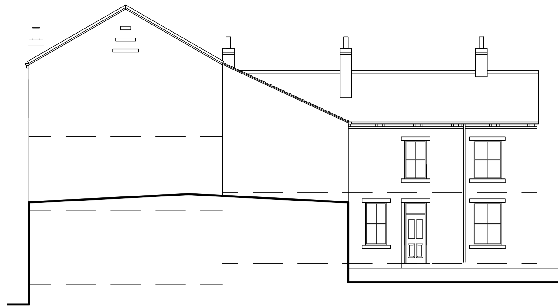
NORTH WEST ELEVATION SCALE 1:100 AS EXISTING
