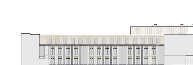
KEY DECISION 08 - Horizontal stone bands and vertical fins added to further articulate the facade and integrate the plant enclosure
