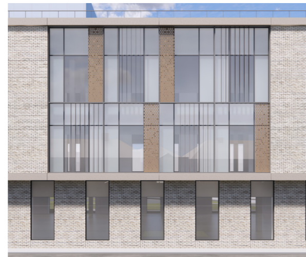
Reconstituted stone band wrapping around first and second floors. Glazed spandrel panels at ground, first and second floors. Cantilever at first / second floor. Large buff brick panels used to break the building into 4 window bays. Perforated metal panels and vertical louvres to provide visual screening from oblique angles.
