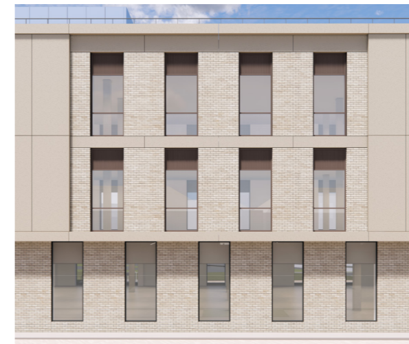
Reconstituted stone band wrapping around first and second floors. Glazed spandrel panels at ground floor only. Cantilever at first / second floor. Large reconstituted stone panels used to break the building into 4 window bays. Decorative metal (bronze coloured) spandrel panels above each window to conceal floor / ceiling build-up. Brick piers between windows at first and second floor.
