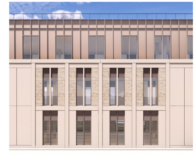
Ground and first floors aligned, second floor set-back. Reconstituted stone zone to ground floor and between bays of 4 windows. Buff brick piers between first and second floors. Decorative metal (bronze coloured) spandrel panels above each window to conceal floor / ceiling build-up. Anodized aluminium panels to second floor. Reconstituted stone / aluminium fins to provide visual screening from oblique angles.
