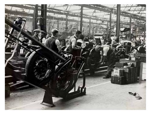
Figure 4.11 Wheels delivered mechanically to assembly line station, 1934 (source: British Motor Figure 4.13 Morris Minor Assembly Line, c.1950 (source: British Motor Industry Heritage Trust) Industry Heritage Trust)
