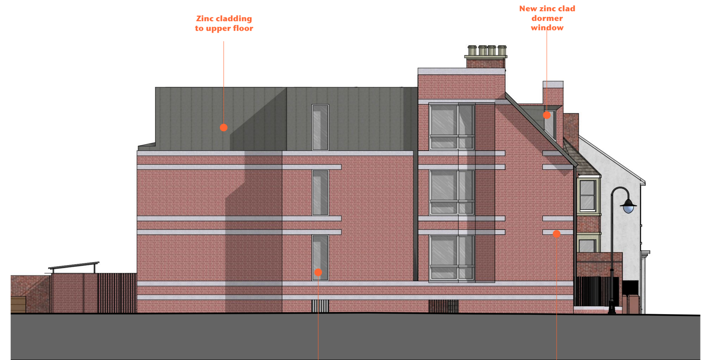
2 East Elevation Housing Block
