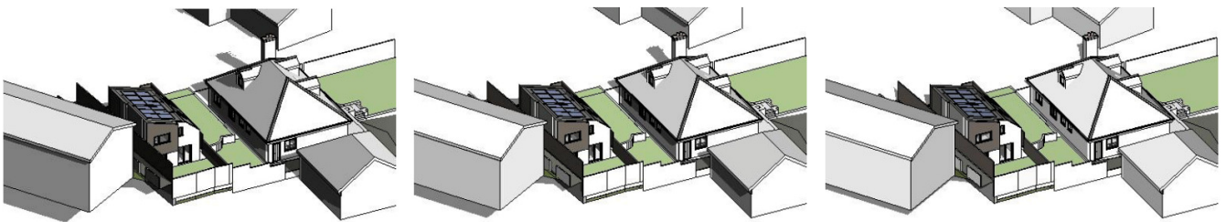
Fig 4: Extract of Solar Study showing the property between 11am-12pm during the Spring Equinox
