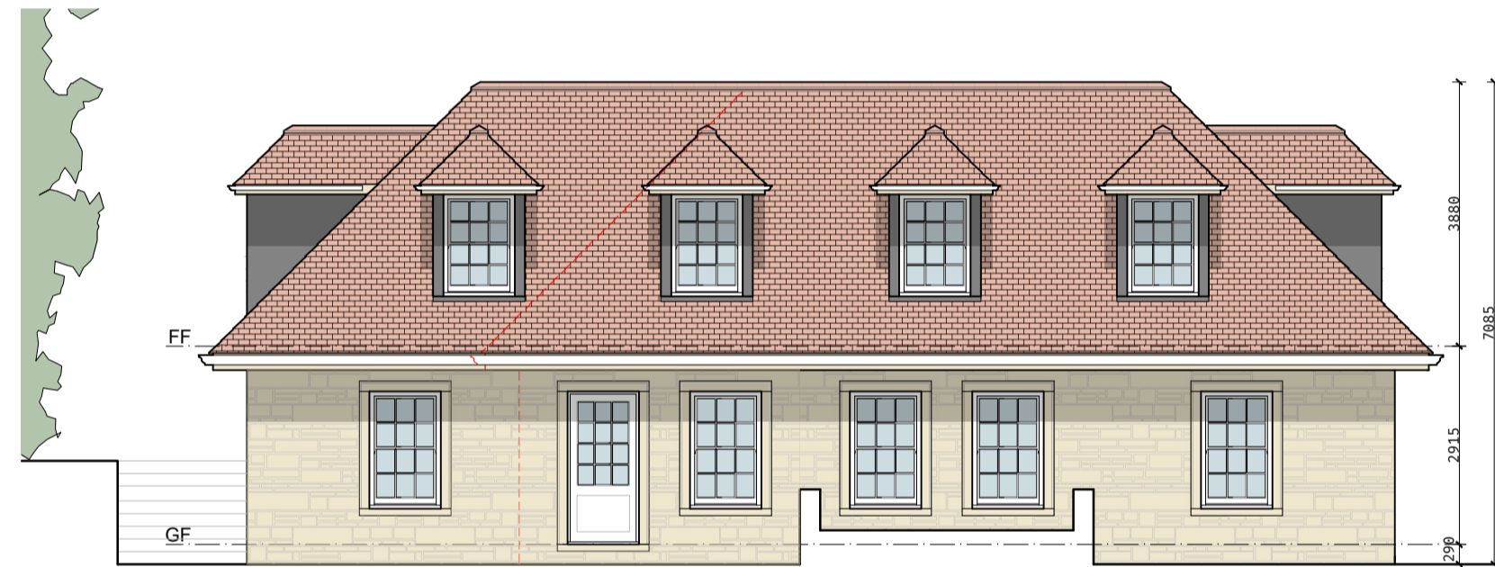
REAR ELEVATION TO TENNIS COURT SCALE: 1:100
