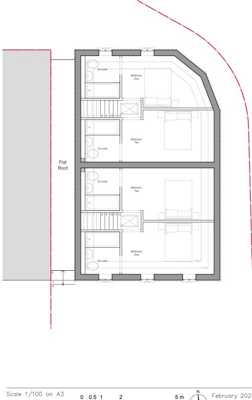
Scale 1/100 on A3 PROPOSED PLANS Ground Floor & First Floor
